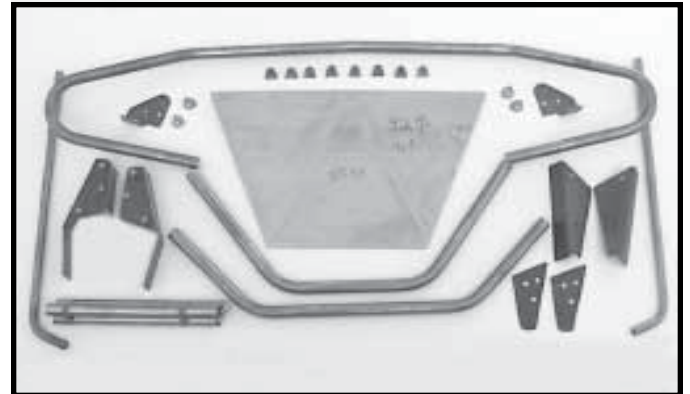
92-96 F150-Bronco Bumper Kit - #FB-9296 Use for 80 to 91 trucks when upgrading to 96 grill
