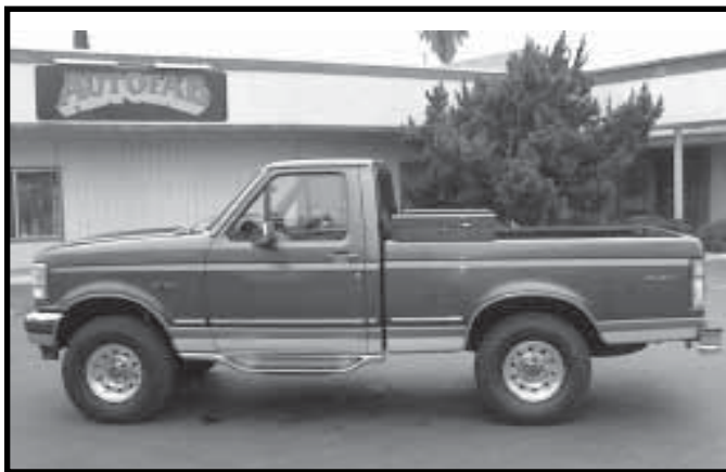
1995 F150 2wd truck with 4 inch econo lift. Rear is stock height Tire size 12.50x33 on original Ford rims
